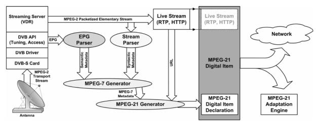
Figure 1 — dvb2di (DVB-to-Digital Item) server architecture.
